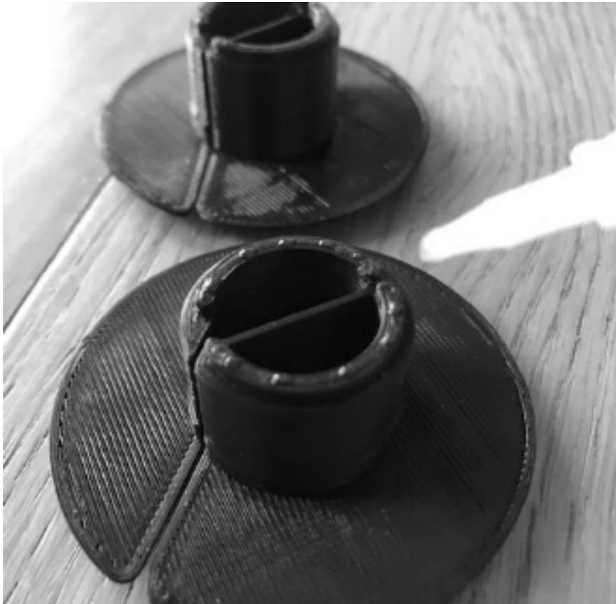
Once ready press each SPOOL A against each SPOOL B (notice that there is a slot to allow the film to be inserted in it. The slot must be well lined up when you assemble the two parts). Keep pressure on it for some time or apply a weight on it so that you can free your hands. for the coming steps.
